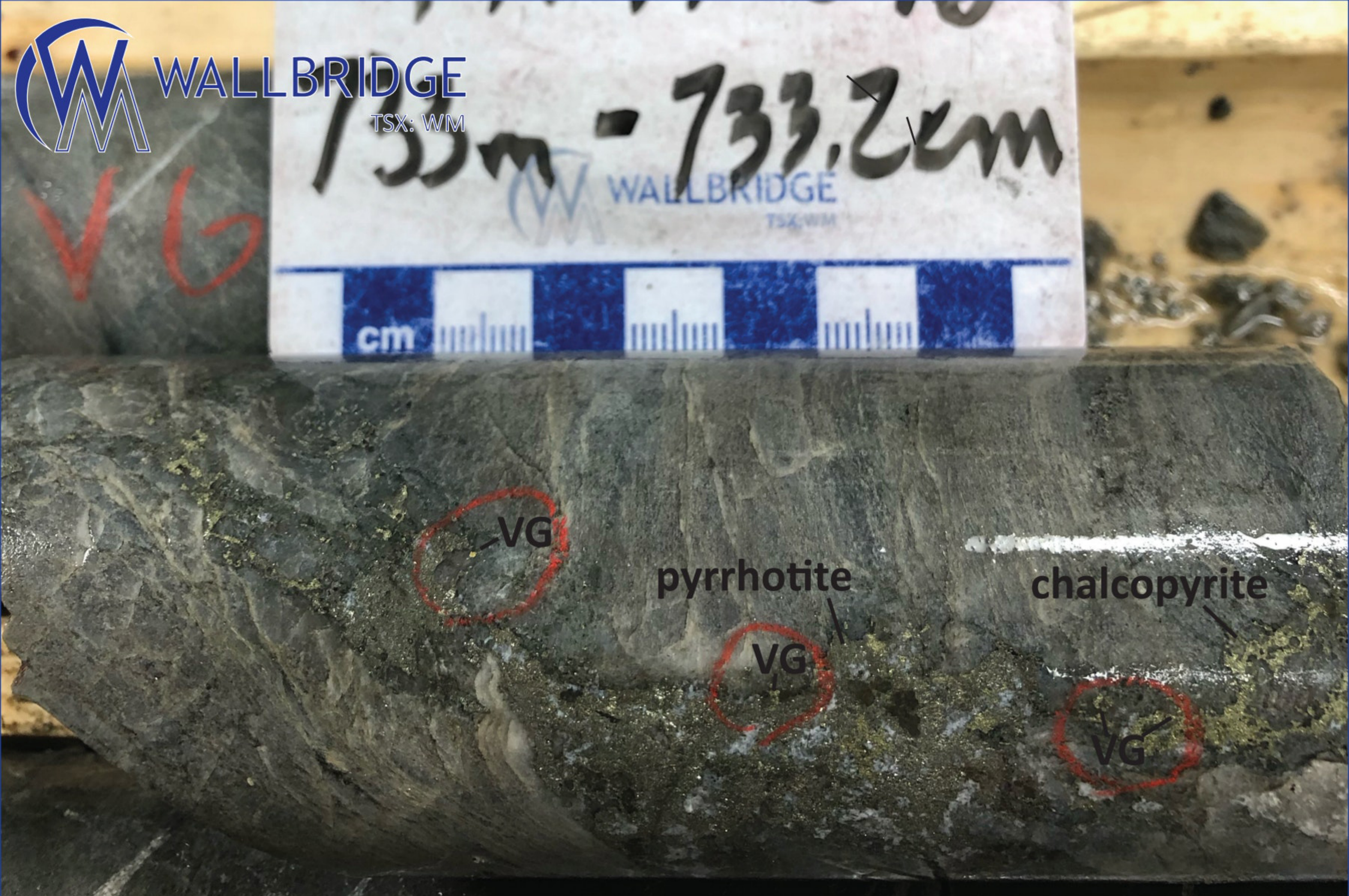
Fenelon Gold - Drill Hole FA-19-096 (733.0-733.2 m): Tabasco Zone Approximately 33-metre core length (723-756 m) with abundant sulfide and visible gold
